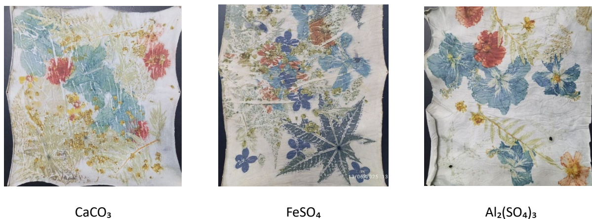
Figure 4. Visualization of Color Difference and Ecoprint Motif on Cabretta Leather Using Three Mordants ( \text{CaCO}_3 , \text{FeSO}_4 , \text{Al}_2(\text{SO}_4)_3 )
