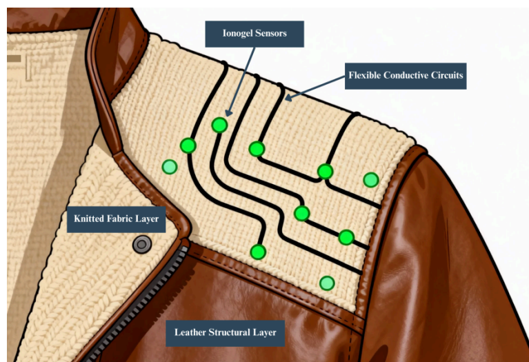
Figure 2. Schematic illustration of an integrated smart sensing system embedded in a textile-leather composite material
