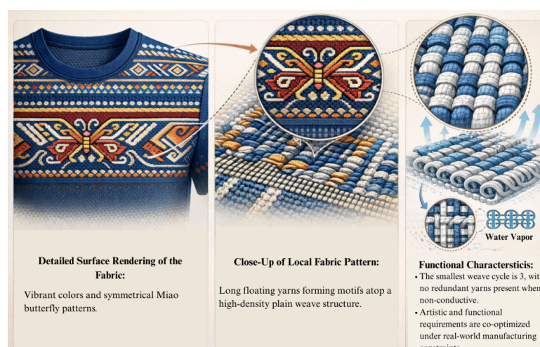
Figure 3. Design and Structure of a High-Breathability Summer Sports T-Shirt Fabric Featuring Miao Butterfly Patterns
