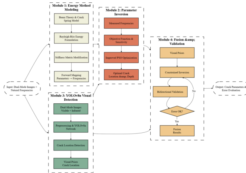
Figure 1. Framework of the proposed multimodal crack identification method
