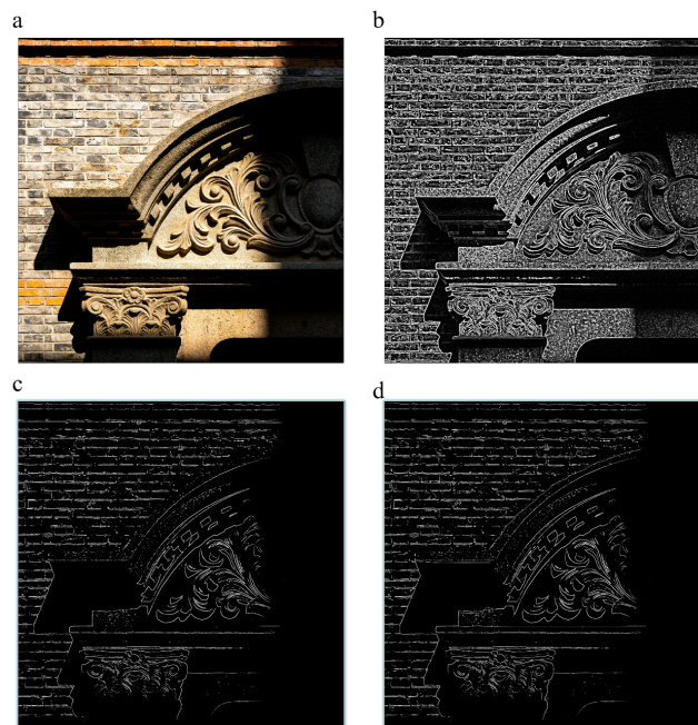
Figure 3. Visual comparison of edge detection operators on Shikumen granite texture: (a) Original grayscale source image showing granular surface noise; (b) Result of the Sobel operator, exhibiting high salt-and-pepper noise due to texture sensitivity; (c) Result of the Standard Canny operator ( T_{high} = 0.2 ), showing significant edge discontinuity; (d) Result of the proposed Optimized Canny algorithm ( T_{low} = 0.05 , T_{high} = 0.15 ) combined with morphological closing, demonstrating superior noise suppression and edge continuity
