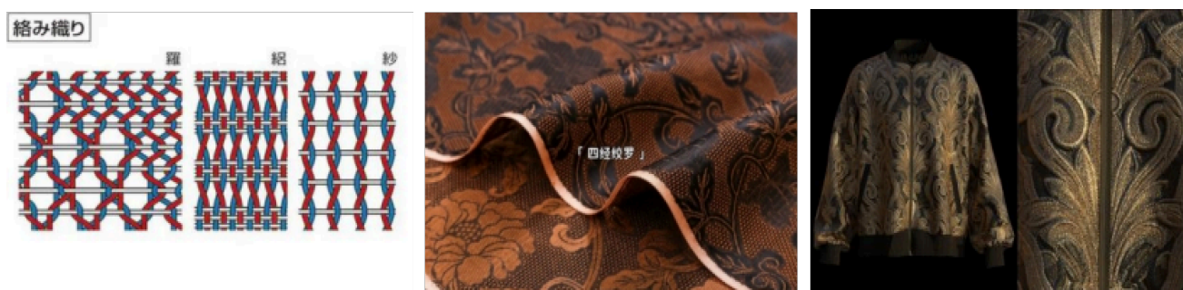
Figure 9. Four-ply warp yarn (four strands of warp yarn) weaving structure (Adapted from: https://image.baidu.com/search/detail )
