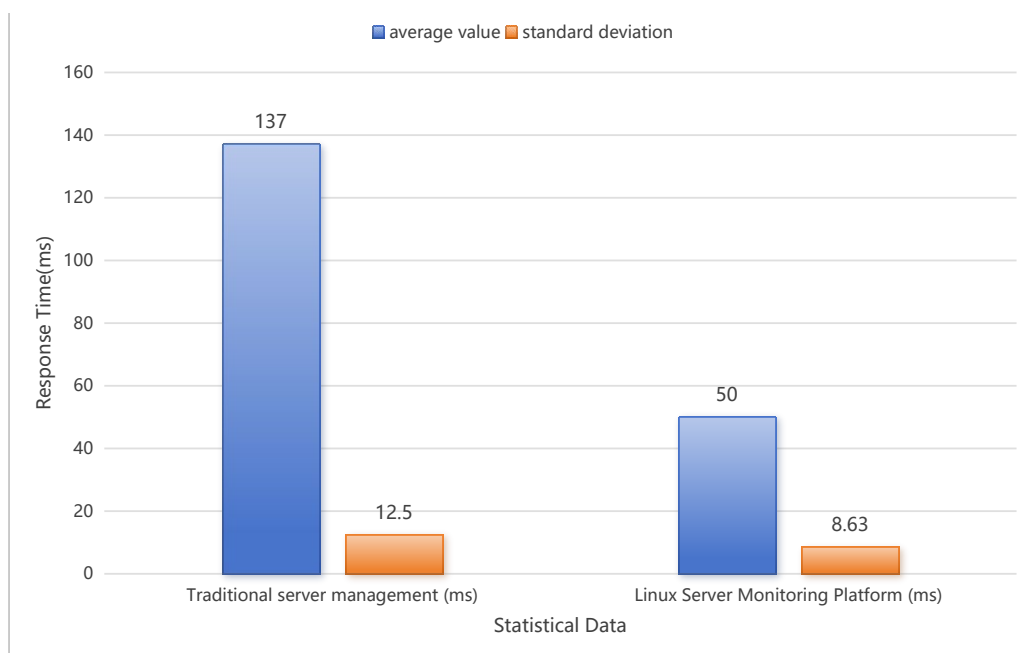
Figure 12. Statistical analysis of response time measurements
