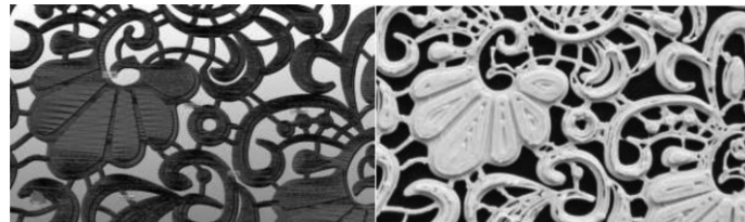
Figure 4. Multi-layer lace pattern, depicted using the Autodesk subsidiary Netfabb GmbH's Software (left panel), and the resulting 3D printed item (right panel) [36]
