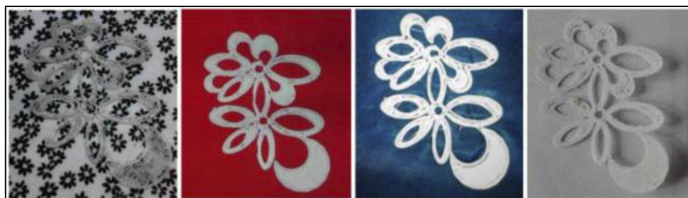
Figure 7. Floral 3DP pattern on cotton, wool, viscose rayon and polyester net textile substrate (from left to right)[36]
