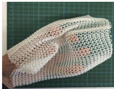
Figure 5. Flexibility of a 3DP weft-knit structure[36]
