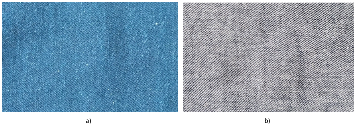
Figure 6. The fabric is made from weft yarn (recycled) containing 50% cotton (virgin) + 50% cotton (recycled) fibre, a) technical face, b) technical backside
