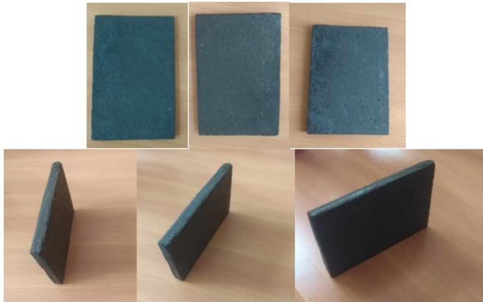
Figure 5. Sisal fibre and wood sawdust reinforced RPET composite sample
