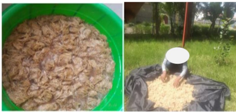
Figure 3. Alkali treatment of sisal fibre
