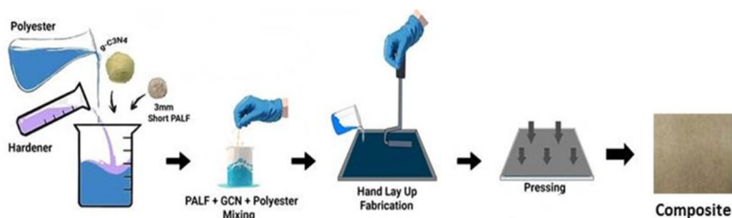
Figure 1. The schematic diagram for PALF reinforced polyester composite using g\text{-C}_3\text{N}_4 filler
