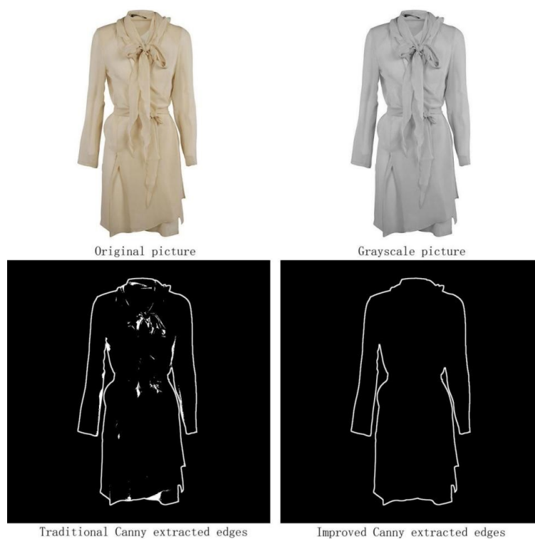
Figure 3. Partial clothing edge extraction results of traditional and improved Canny algorithms
