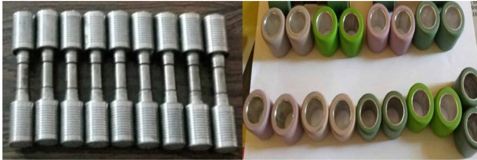
Figure 2. Roller bar shells after mounting and different degrees of rubber cots
