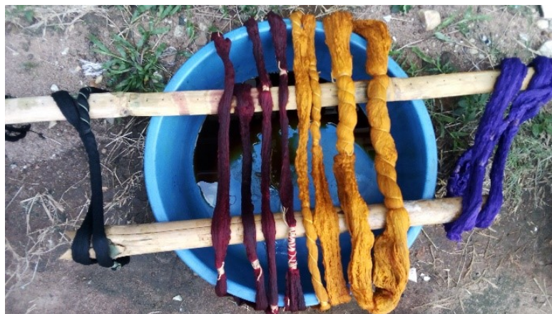
Figure 6. Oxidation of the dyed warp yarns
