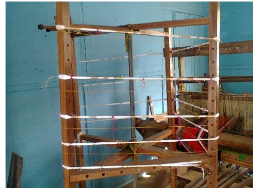
Figure 2. Tying of the warp yarns at the various sections of the warp
