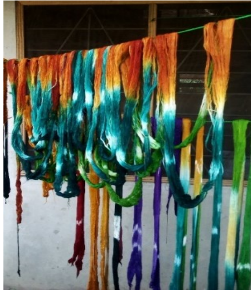
Figure 7. Drying of the Ikat dyed warp yarns after the excess dye was washed
