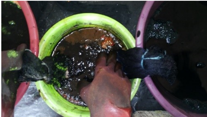
Figure 5. Dyeing of the warp yarns using the Ikat technique with three colours concurrently
