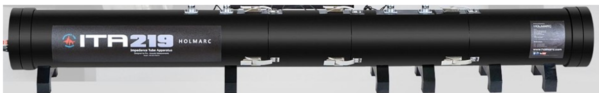
Figure 1. Impedance tube method used for measuring normal incident sound absorption coefficient [21]
