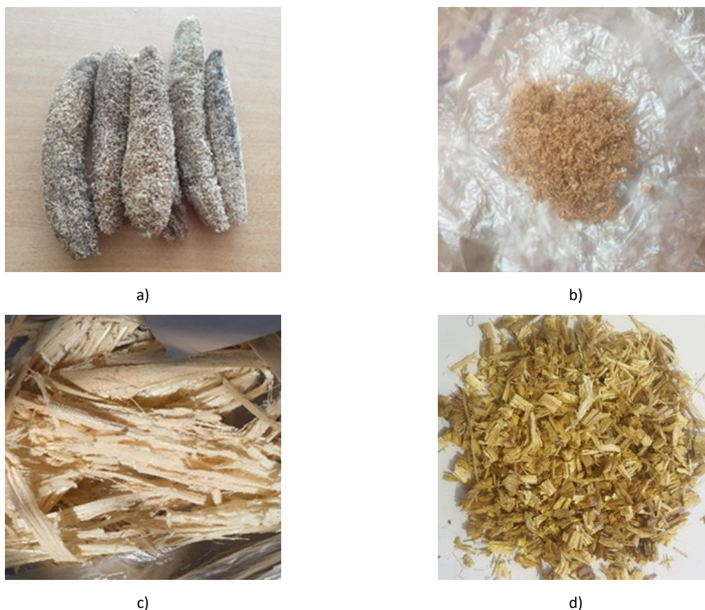
Figure 1. Reinforcement material a) luffa; b) cut luffa fiber; c) raw bagasse fibers; d) cut bagasse fiber
