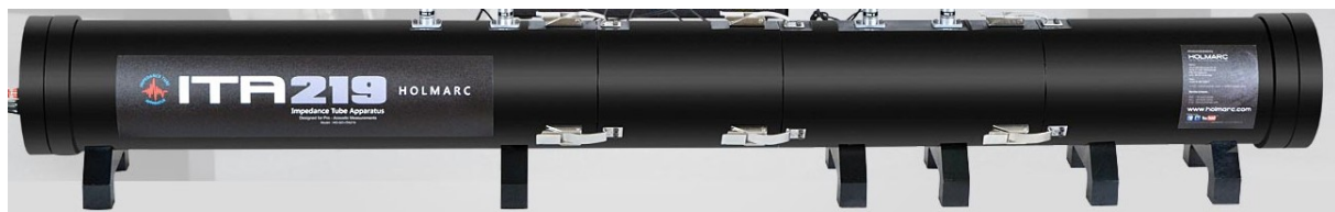
Figure 1. Impedance tube used for measuring sound absorption coefficient
