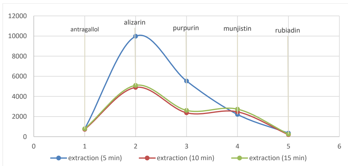
Figure 2. Identified dyestuffs and their peak (heights) in the extractions
