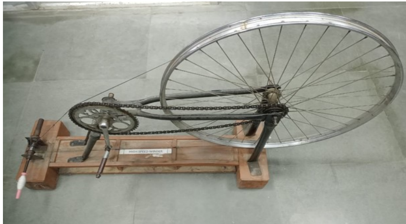
Figure 12. High speed winder used in handloom sectors
