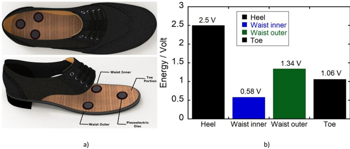
Figure 5. (a) Positioning of piezo disc in different position (b) Generated energy (Volt) at different portion
