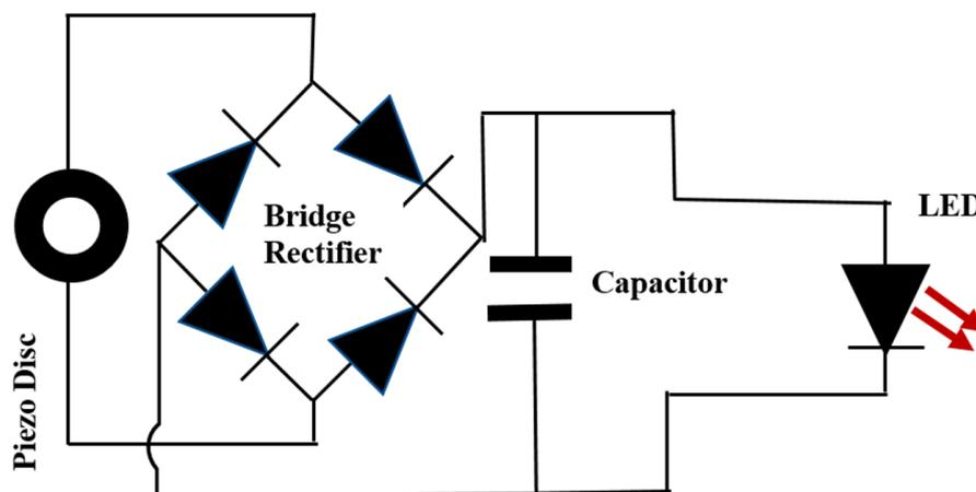
Figure 3. Schematic drawing of piezoelectric energy harvesting
