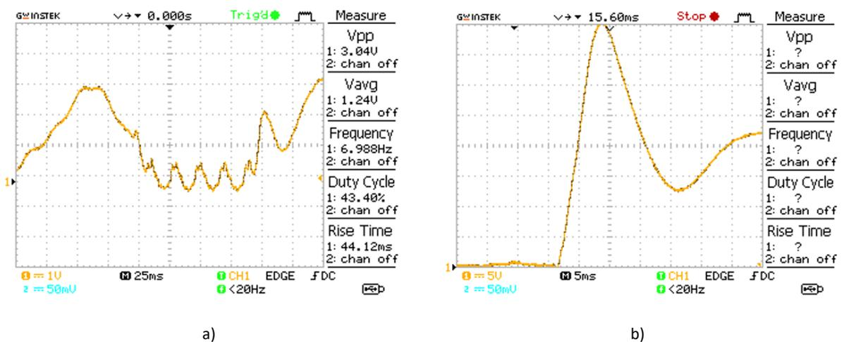
Figure 4. Waveform shape for pulsating (a) DC 3.04 V; (b) DC 23.2 V
