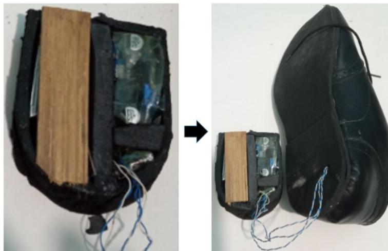
Figure 1. Inserted circuit at the heel portion and complete preparation for sole and heel attachment
