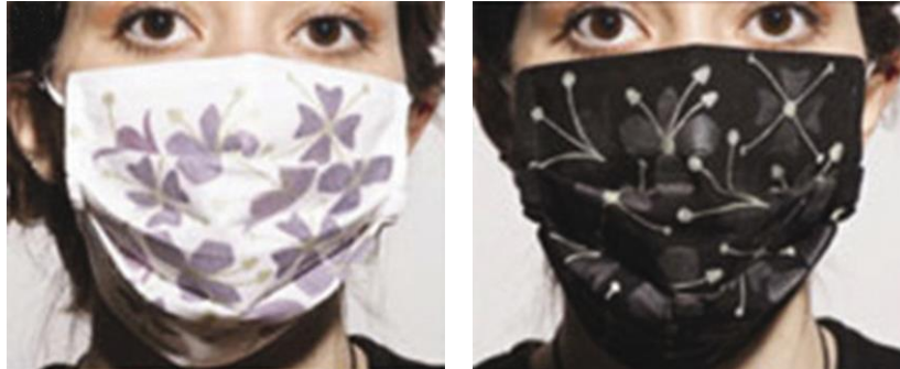
Figure 10. Colour change due to thermochromic print highlighting floral print on white background by changing from black colour when heat is supplied [22]
