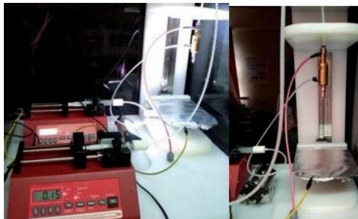
Figure 2. The photo of electrospinning experimental set-up used to prepare silk fibroin nanofibers from aqueous formic acid solution of regenerated silk fibroin (foam) and olive leaf extract
